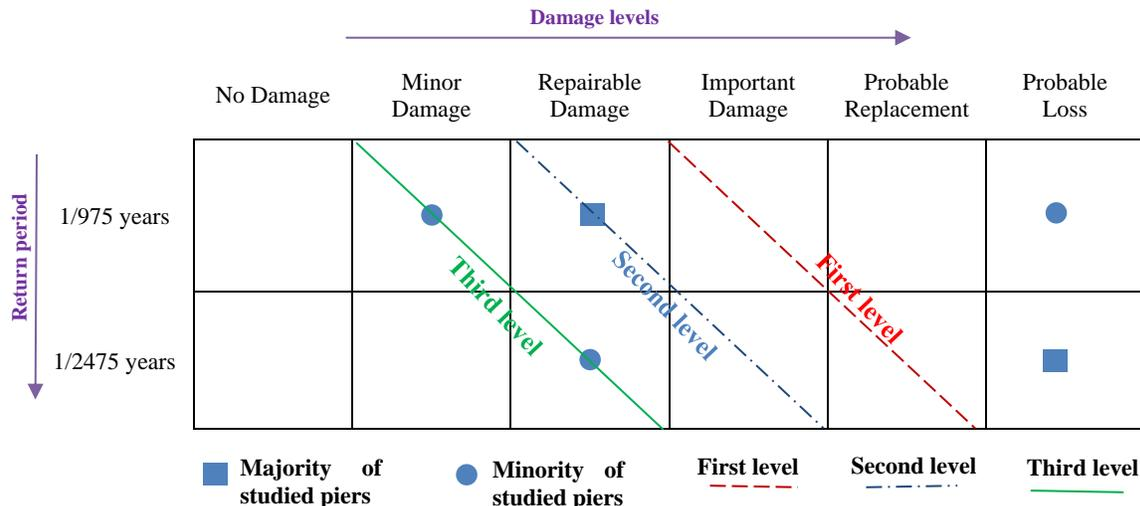
Figure 5. Piers Seismic performance according to the engineer's evaluation
