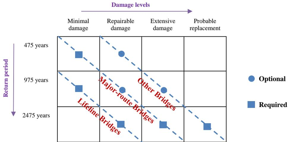
Figure 4. Bridge damage levels for different return periods according to CSA-S6-14
