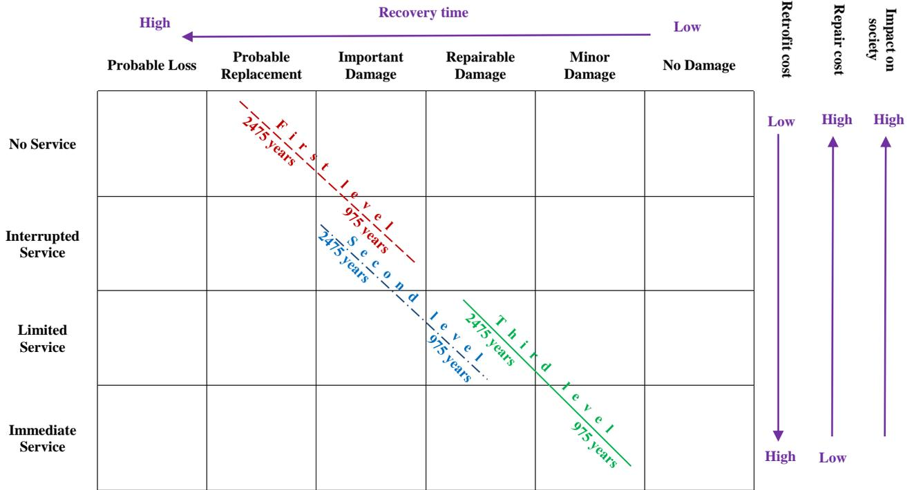
Figure 6. Three seismic retrofit levels of the Jacques Cartier bridge
